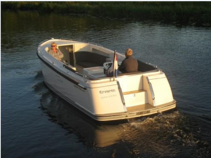
An open stern makes it easy to board and features a removable seat back for even better access to the swim platform. The self-draining cockpit has three large drainage points and one part of the flooring is hinged to the engine casing, which also contains a cooker, to allow immediate access to the engine.
