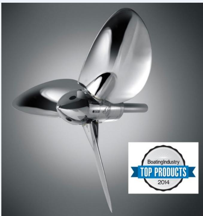
The blades of "EWOL Hi-Speed" have been designed specifically to have a center of thrust rearmost so as to create a fin effect that keeps the propeller in the feathering position in any condition, even when the water flow is disturbed by the effect of the hull appendices in water at high speed.
