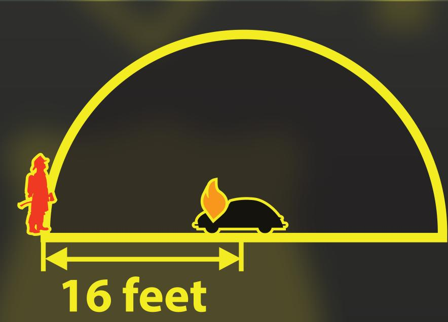
First Responders may effectively and safely control the fire around the battery pack from a defensive position while allowing the battery to burn itself as the sealed battery pack is nearly impossible to extinguish.
