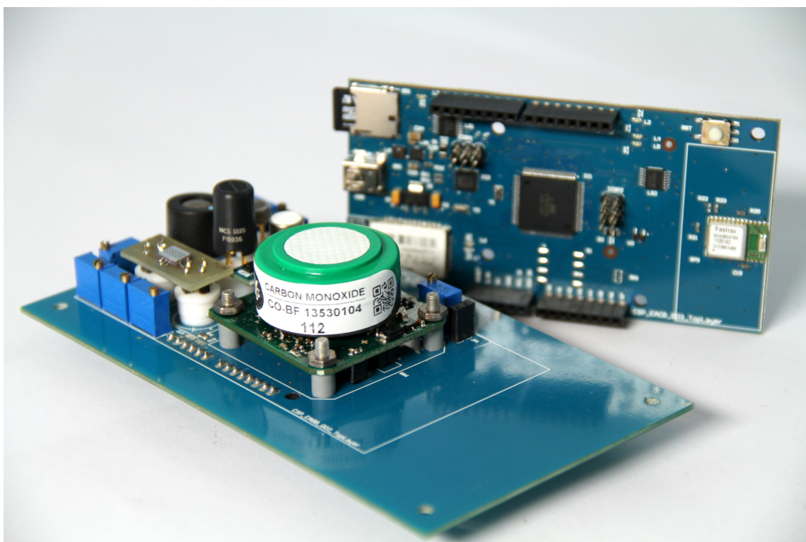
Figure 6: Sensing device. The two electronics boards of the sensor box with the gas sensors mounted on top of the sensor shield.
