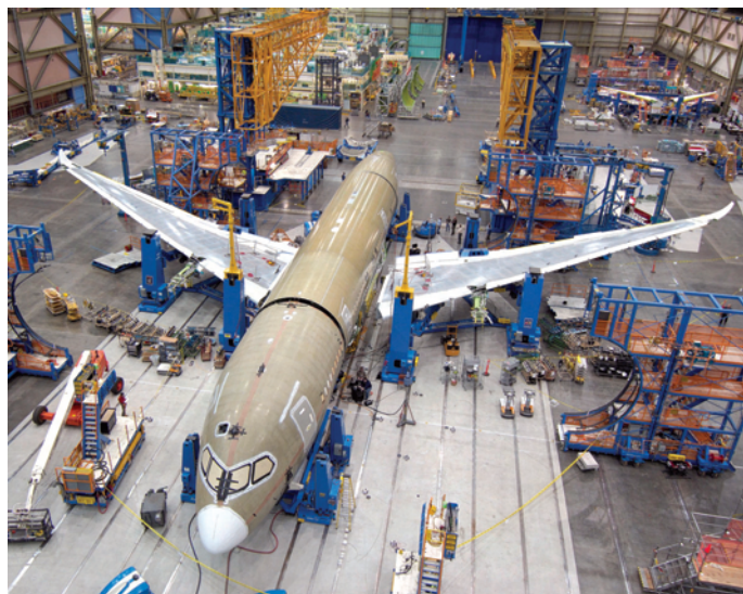
Final assembly begins on fifth Boeing 787 Dreamliner. Each Dreamliner will contain more than 250,000 pounds of titanium. Photo courtesy: The Boeing Company
