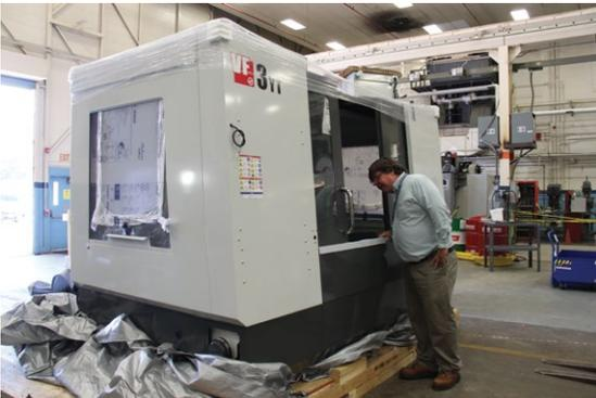
HAAS VF 3 YT vertical machining center.
