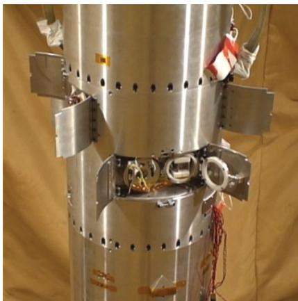
Ampoules visible in payload after door deployment.
