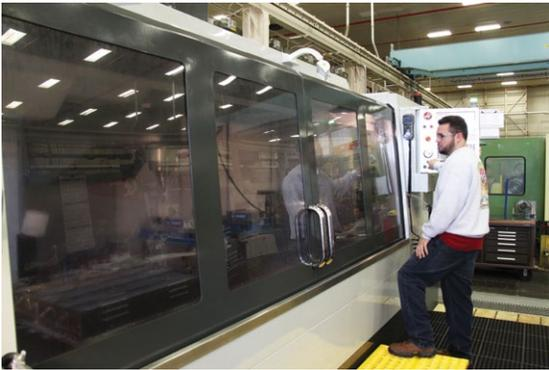
HAAS VF11 vertical machining center.
