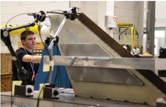
NSROC Testing and Evaluation group intern, Seth Austin, conducting a fin bend test.
