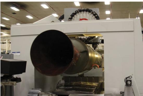
Taurion motor casing being modified in the machine shop.
