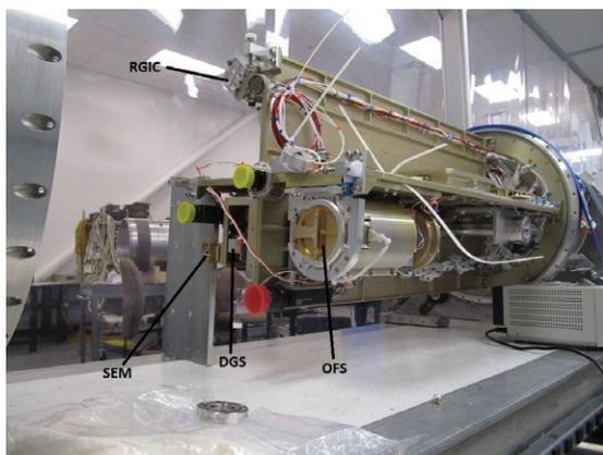
Degradation Free Spectrometers science payload
