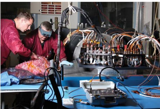
Vibration testing of the WFF Avionics Pallet for LDS.
