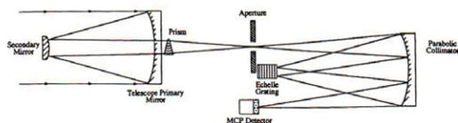
Geometry of the VeSpR telescope and spectrograph.
