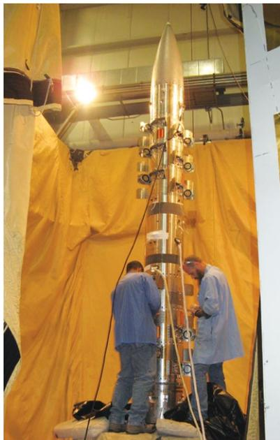
C-REX payload with doors deployed.
