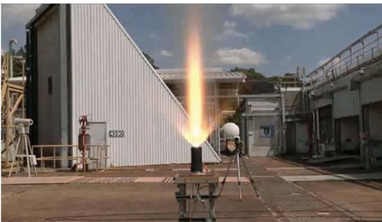
Open air Peregrine igniter test at Marshall Space Flight Center.
