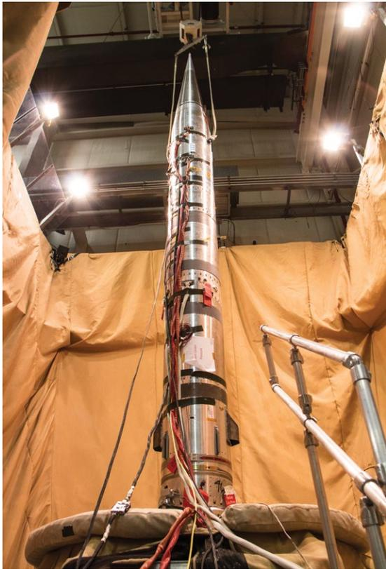
The Sub-TEC 6 payload during deployment testing at Wallops.
