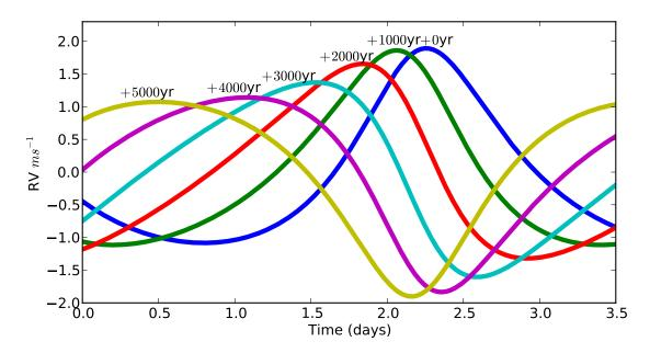
FIGURE 1. This diagram shows how the shape of the radial velocity curve of XO-3b [4] changes over time due to relativistic precession. Every 1000 years, the argument of pericenter advances by 40 degrees.
