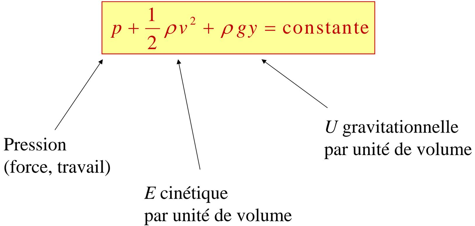
The diagram features a central yellow box with a red border containing the Bernoulli equation. Three arrows originate from text labels below and point to specific terms in the equation: one from 'Pression (force, travail)' to the pressure term 'p', one from 'E cinétique par unité de volume' to the kinetic energy term '1/2 rho v^2', and one from 'U gravitationnelle par unité de volume' to the potential energy term 'rho g y'.
